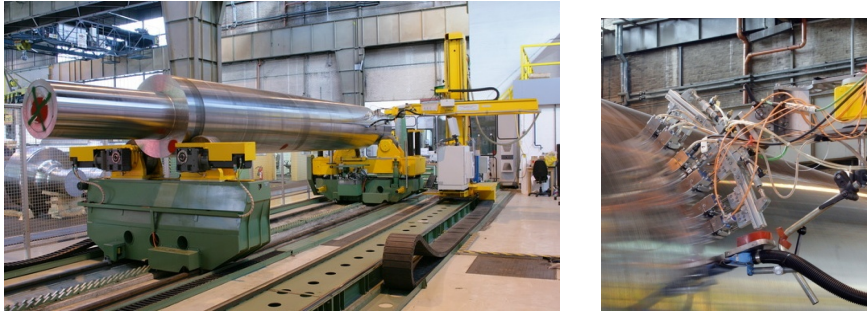
FIGURE 6. Shaft inspection facility (2007) and six unit probe holder.
